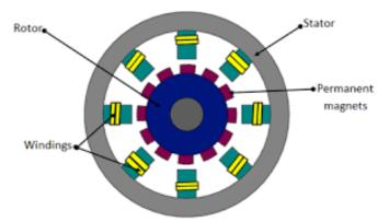
can easily rotate at the frequency of the input power supply, i.e., both the rotor frequency and that of the input power supply are same. These motors are classified as Permanent Magnet Synchronous Motors or PMSM. Thus the PMSM does not have any losses in the rotor due to the slip.
